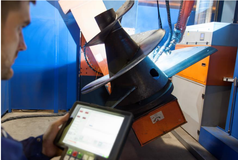
Caption 9: Precision during the manufacture of the core component in every mixer wagon - robots weld the different parts that make up the mixing auger.
