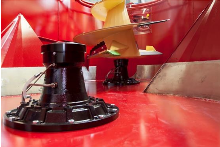
Caption 5: Forming the “core” of every mixer wagon, the mixing augers are inserted with utmost care during final assembly.
