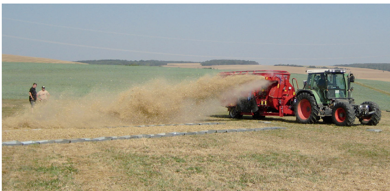
Figure 5: Straw distribution at a throwing distance of 15 m
