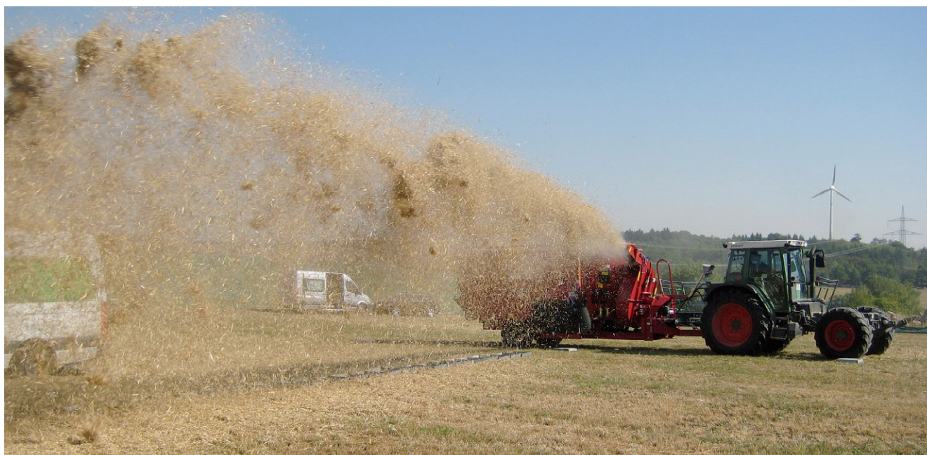
Figure 4: Straw distribution at the maximum throwing distance
