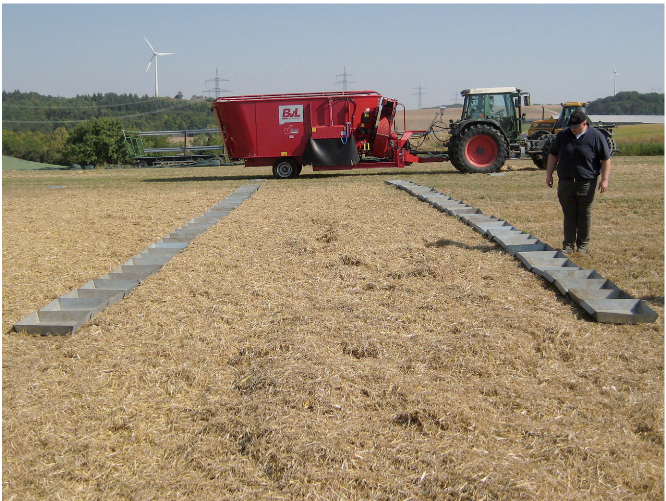
Figure 3: Measurement of the straw distribution using collection trays
